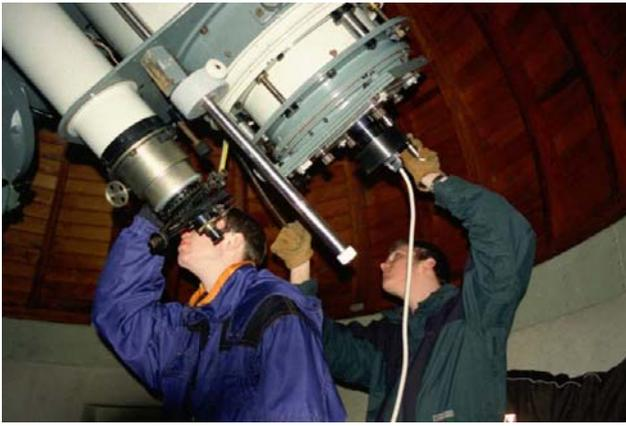
**Fig. 6:** The Bolivia Astrograph is prepared for CCD observations with a ST6 camera
